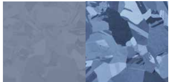
textured wafer vs. polished wafer after 4 \mu\text{m} etch depth
